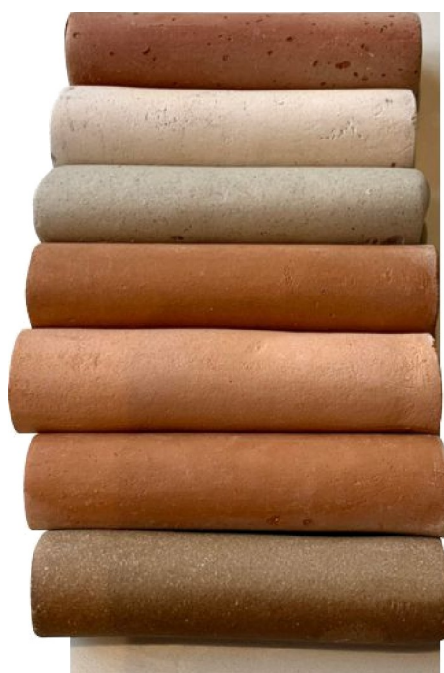
Figure A - Ceramics obtained through different production techniques (different raw materials and firing at different temperature gradient). Below, the ceramic specimen representative of the TAVA amphorae under study
